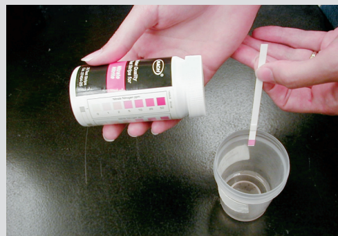
Figure 4-2. Nitrate and nitrite test strips are easy to use. Simply dip in the water and then record the color change after about two minutes.
