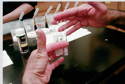
Figure 4-3. The ammonia test strips have a compound on the test strip that reacts with ammonia to cause the color change. Strips react within a vial of sample water for 30 seconds and can be read after another 30 seconds
